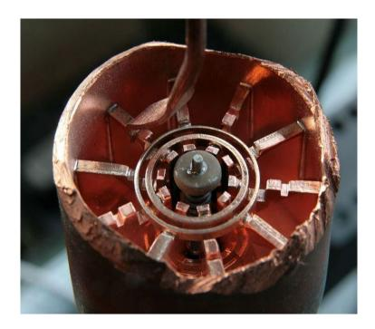
Figure 8. Magnetron cut open to show the cavities. By placing metal tabs inside the cavities, we can increase the frequency output. You do not want the magnetron operating at 2.45 GHz, because the atmosphere (water) will absorb most of its energy.
