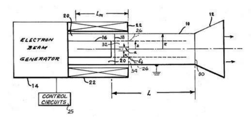
Figure 4. From Patent 4345220 for a Vircator microwave weapon.
