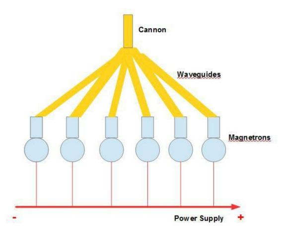
Figure 7. Microwave cannon basic design, consisting of car batteries, magnetrons, waveguides, and associated wiring that makes each magnetron fire at the same time. The focusing magnets should be sized for 1/6 wavelength. In other words, if the wavelength is 6 inches, size the hole in the focus magnets for 1 inch.
